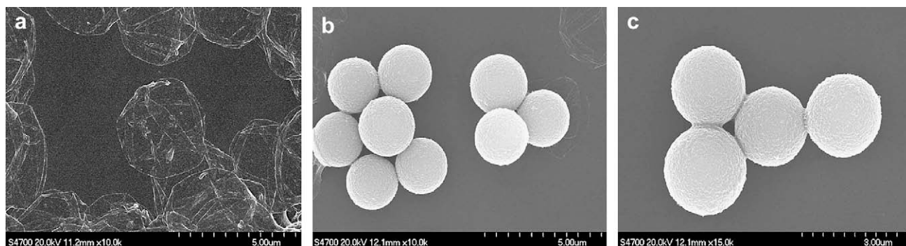
Fig. 1. SEM images of the (ALG/CHI) 5 hollow shells (a) and shells upon incubating the preformed shells in various organic solutions in pure water medium: (b) DCP; (c) SA. Scale bars are 5 \mu\text{m} for a, 5 \mu\text{m} for b and 3 \mu\text{m} for c.
